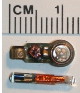
Figure 2.1. PIT tag (bottom) and JSATS dual-battery configuration acoustic transmitter (top) size comparison
